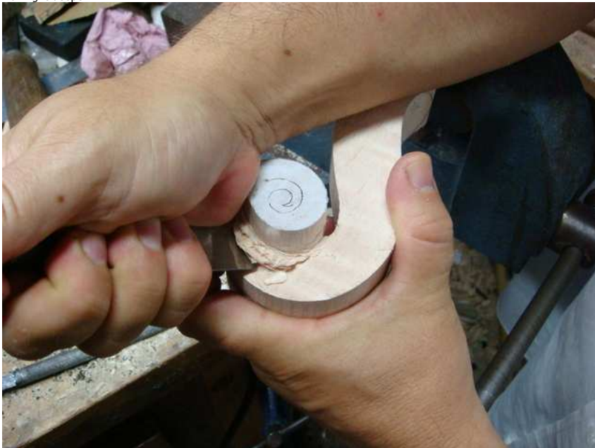
Correcting the curves with a small sculptor's curved rasp:
