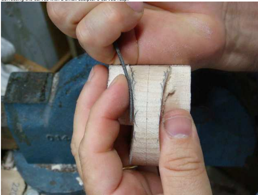
Now the front view. The scroll is tridimensional, so allways check it visually in different angles while you are working, front view and side view mainly. The lines most flow harmoniously without hills and valleys:
