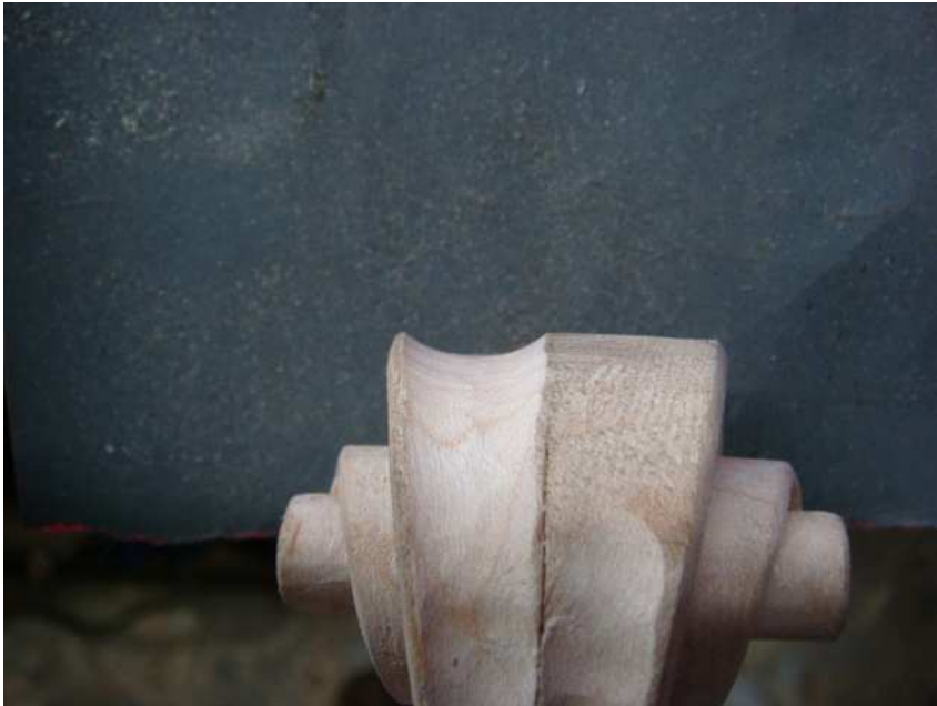
Here Im working in the fluting in the throat region with a knife:
