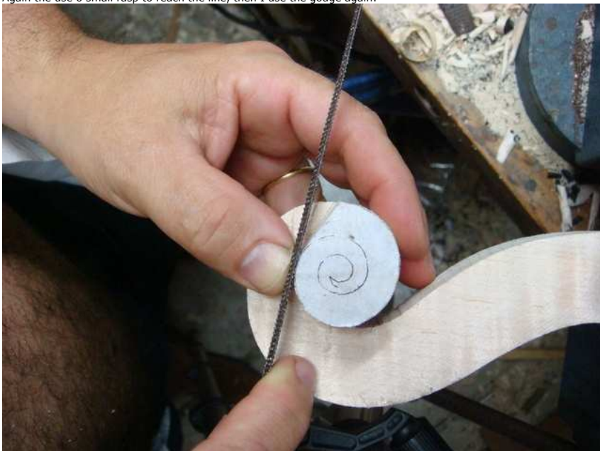
Again the use o small rasp to reach the line, then I use the gouge again:
