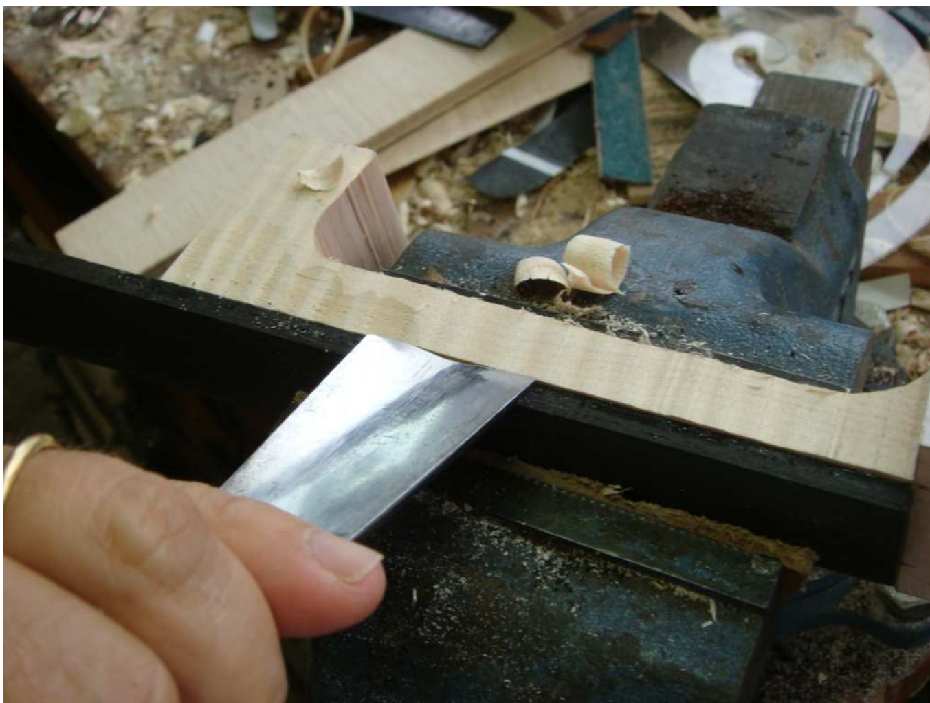
Here I'm working in the neck root part with a wide Japanese chisel (nami)
