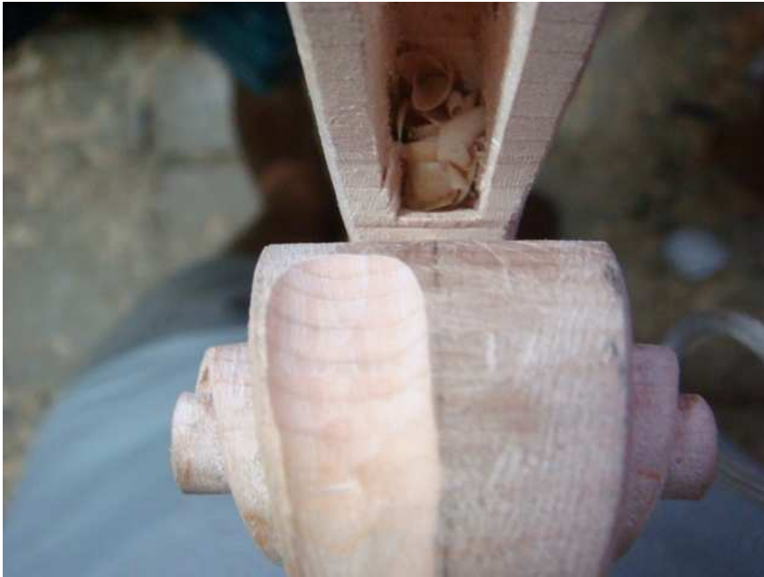
Here a view of the fluting of the front part of the scroll. I put a piece of sandpaper on the back to give contrast:
