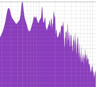
The highest peak shows up at 486 Hz. As a check to make sure this is A1 and not B1+, the same test was performed with the microphone at the upper area of the F-hole... and the peak all but disappeared. This is what should happen for A1, but not for B1+.
