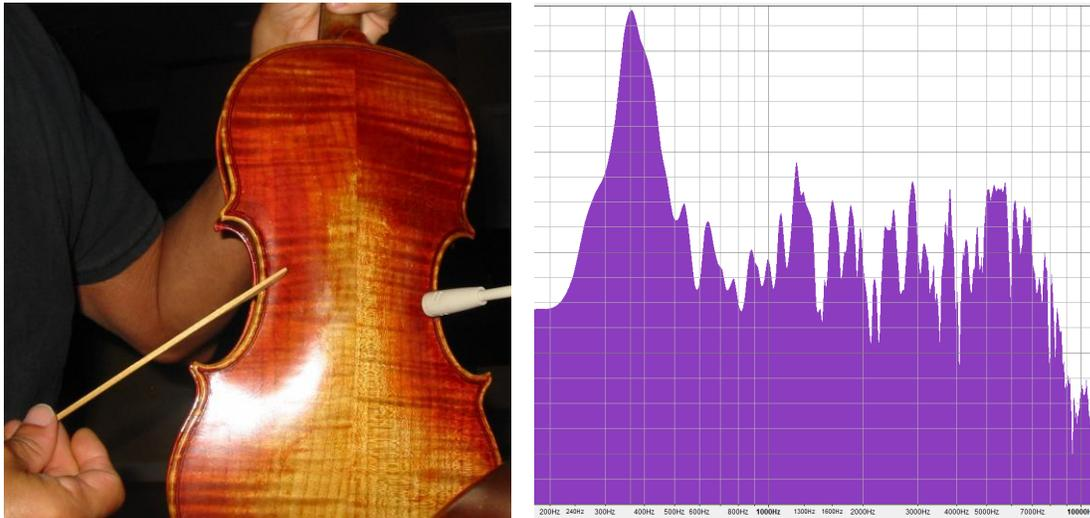
There's no mistaking the peak of the spectrum at 360 Hz.
