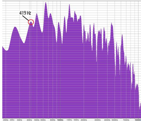
Now we find a modest peak at 419 Hz, which is most likely the actual B1- mode. It is likely that the weakness of this mode and the strong nearby CBR mode combined to show the small peak at 400 Hz in our initial measurement.
